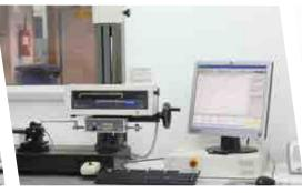
Roughness tester / CNC contour measuring instrument ZEISS TSK Surfcom 1800 D-23-N
