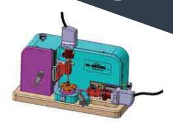
Inside control station for holes by means of fiber optic visor
