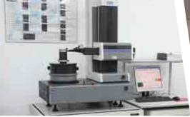
ZEISS TSK Rondcom 60 cnc rotational accuracy form tester
