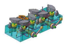
Multiple pallet for machining centre with manual workpiece positioning and hydraulic clamping
