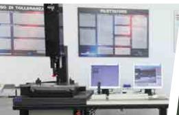
MICRO-VU 3D CNC optical QUIBIC series measuring machine
