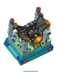
Pallet for Grob machining center with workpiece clamping from above
