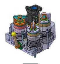
Turret for machining center with manual workpiece positioning and hydraulic clamping
