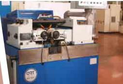
Thread rolling machine ORT RP 30/U
