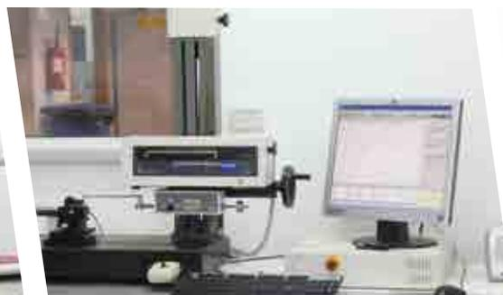
Roughness tester / CNC contour
