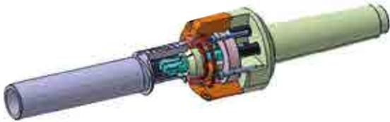
Tailstock with phasing/driving system on inside grooved profile by means of an expander
