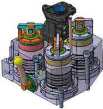
Turret for machining center with manual
