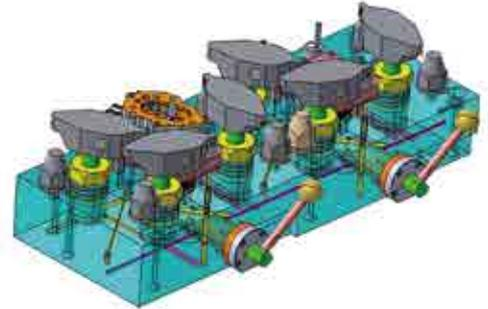
Multiple pallet for machining centre with manual workpiece positioning and hydraulic clamping
